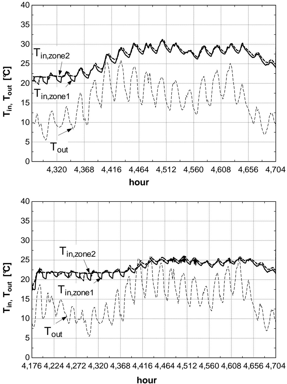
Fig. 8.2: Indoor temperatures computed in both Esneux house zones, with corresponding outdoor temperatures, for a **mean summer**, without comfort improvement strategies (up) and with controlled external blinds and free cooling by opening windows (down).
