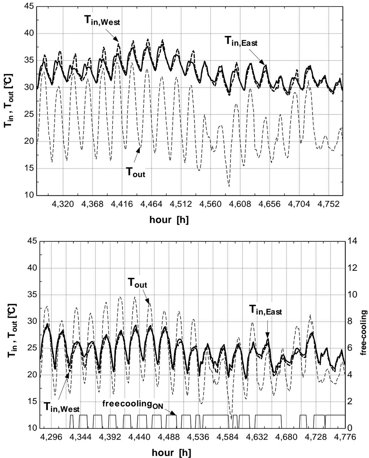
Fig. 8.7 Indoor temperatures computed in the East and West ground floor offices, and corresponding outdoor temperatures, for a summer hot wave, without comfort improvement strategy (up) and with stack free-cooling and controlled blinds (down).
