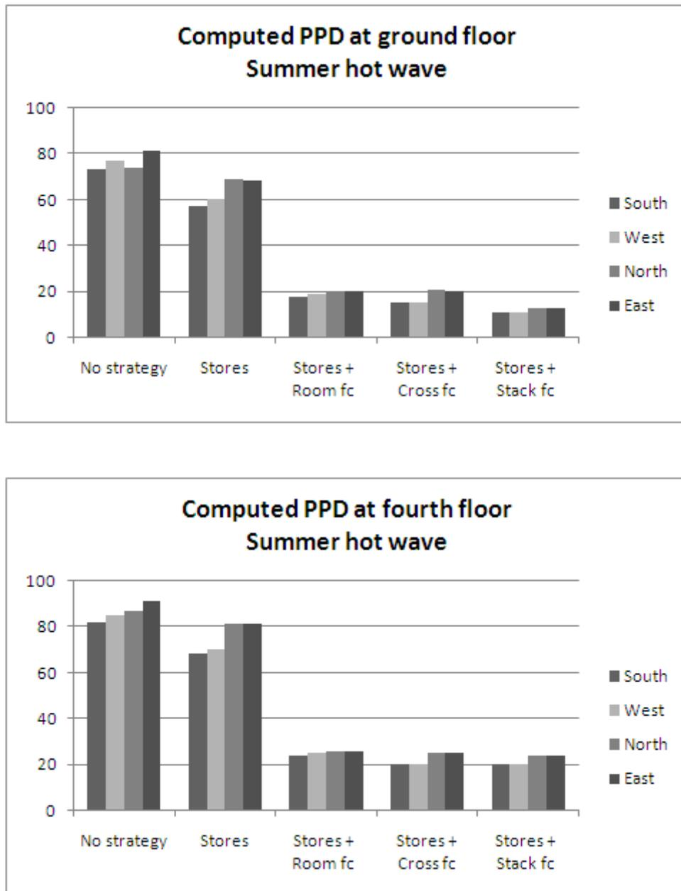
*Fig 8.6 Predicted Percentage of Dissatisfied related to different office orientations and to different natural free cooling strategies, for a summer hot wave, at ground floor (up) and at fourth floor (down) of a four levels office building.*
