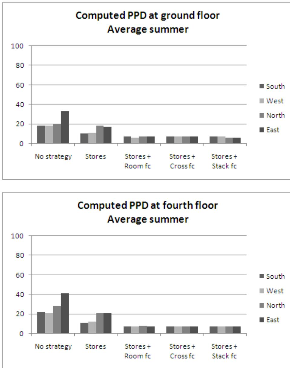
Fig 8.5 Predicted Percentage of Dissatisfied related to different office orientations and to different natural free cooling strategies, for an average summer, at ground floor (up) and at fourth floor (down) of a four levels office building.
