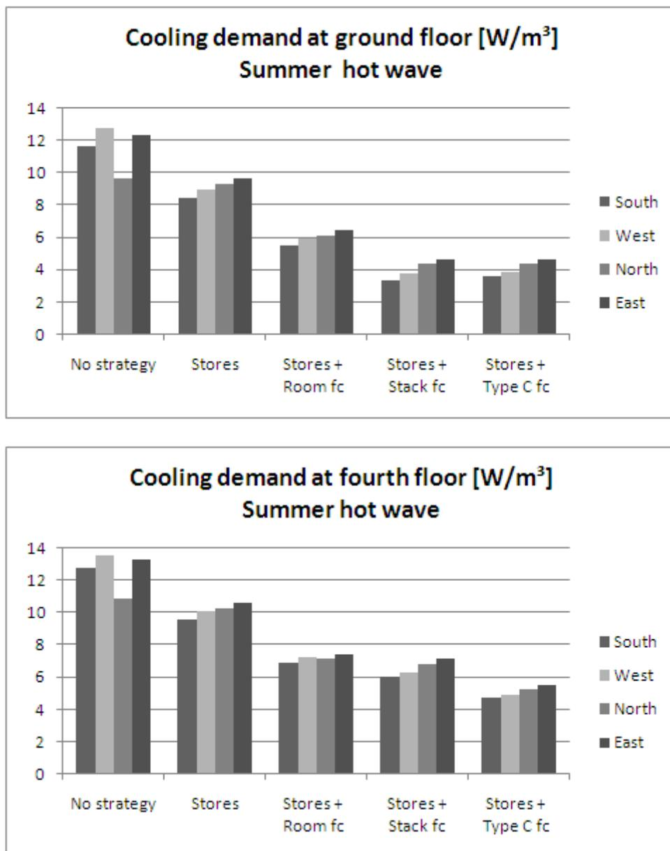
Fig 8.10 Cooling demands per m<sup>3</sup> of conditioned space, related to different office orientations and to different natural free cooling strategies, during occupancy hours for a summer hot wave, at ground floor (up) and at fourth floor (down) of a four levels office building.
