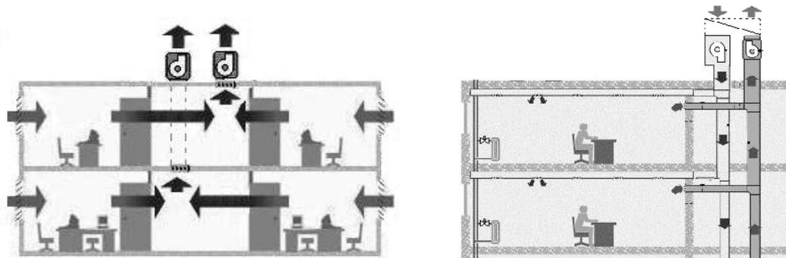
Fig 8.8 Combined natural and mechanical free cooling strategies in office buildings: system C (left) or D (right).
