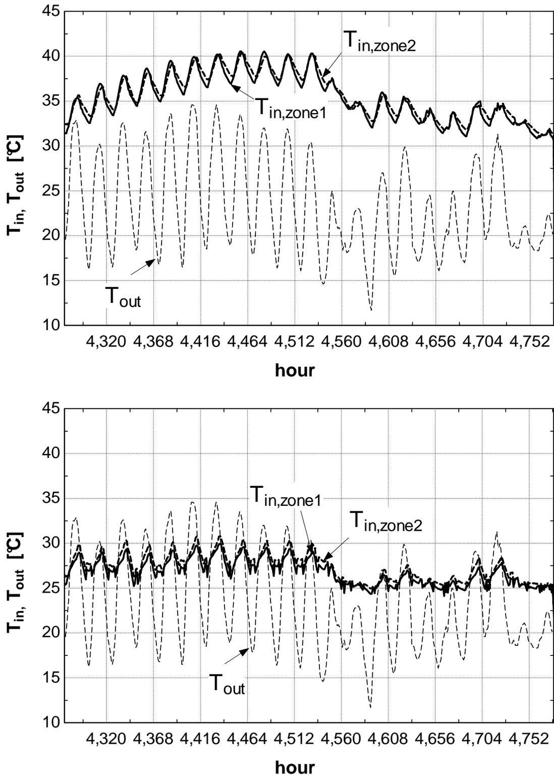
Fig. 8.3 Indoor temperatures computed in both Esneux house zones, with corresponding outdoor temperatures, for **1976 summer hot wave**, without comfort improvement strategies (up) and with external blinds and free-cooling by opening windows (down).
