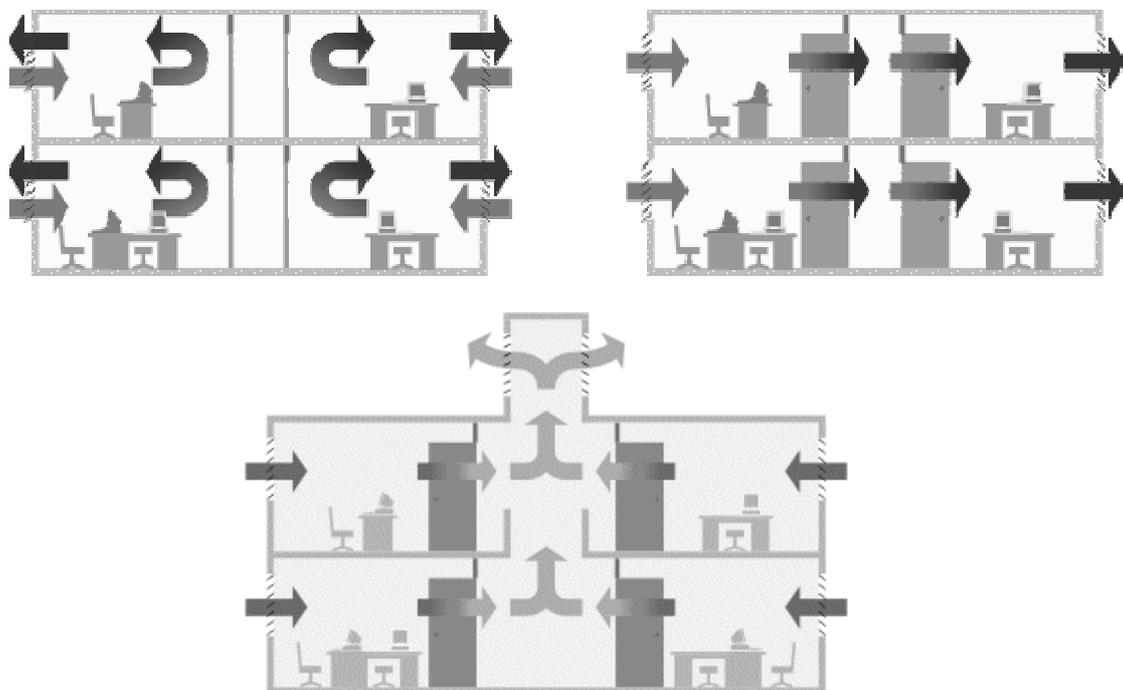
Fig. 8.4 Natural free-cooling through room free-cooling (left), cross free-cooling (right) or stack effect (below) [39].
