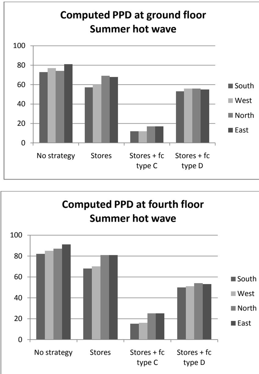
*Fig 8.9 Predicted Percentage of Dissatisfied related to different office orientations and to different natural free cooling strategies, for a summer hot wave, at ground floor (up) and at fourth floor (down) of a four levels office building.*
